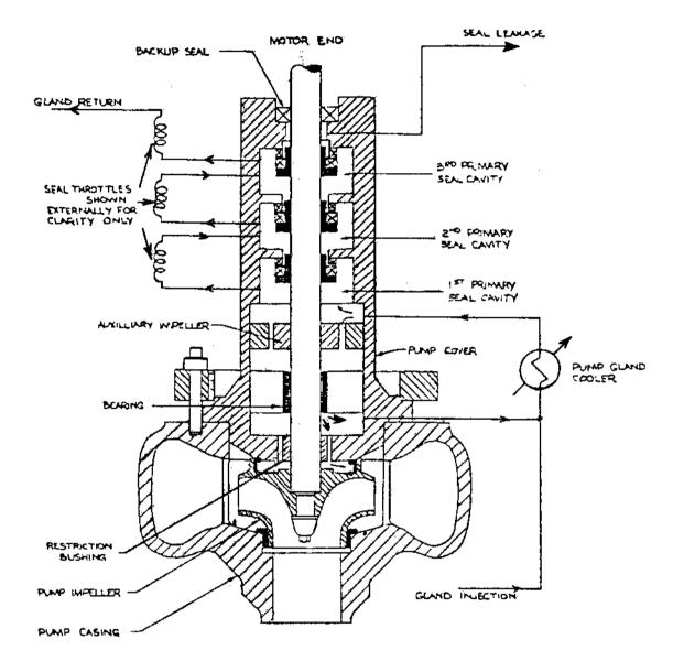
Figure 2: Simplified HT Pump Gland
